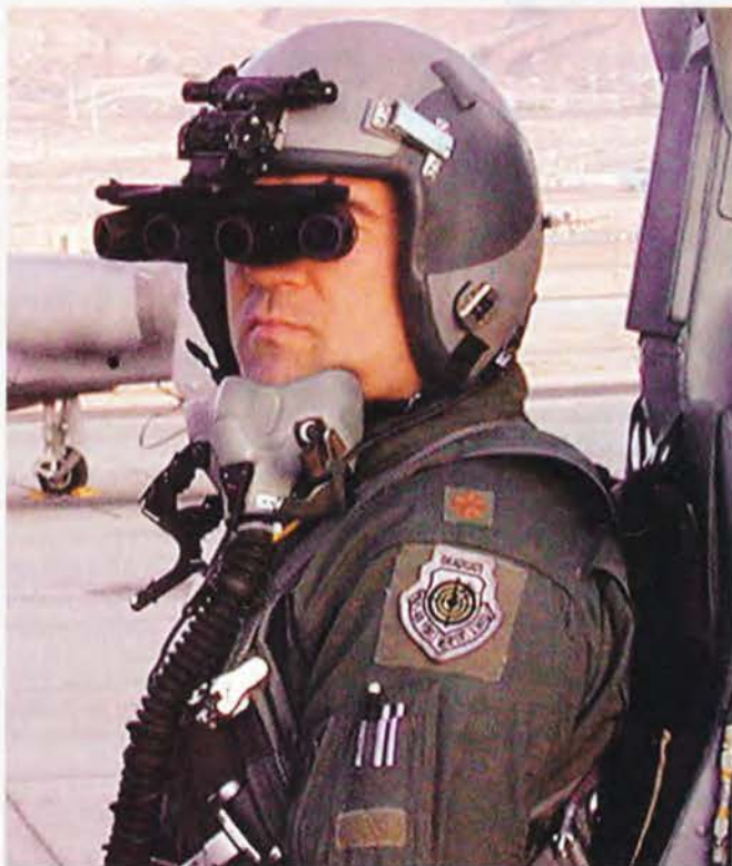
Panoramic Night Vision Goggles will give pilots a 95-degree field of view — more than double the current 40 degrees.
